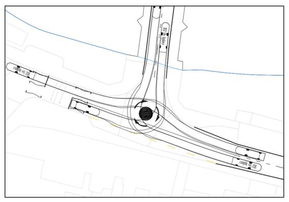
Figure 6 Indicative Mini-Roundabout Layout for Site 1
